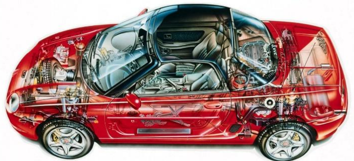
Cut away image of the 1995 MGF showing the running gear used in the Mini
