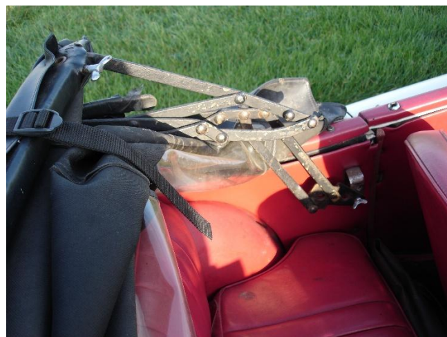
The hood mechanism is a little intrusive for anyone in the back but allows the hood to fold behind the rear seat
